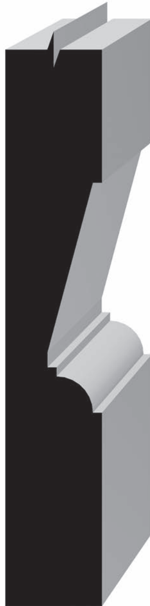
1" Thick Traditional Raise with Ovolo Sticking
