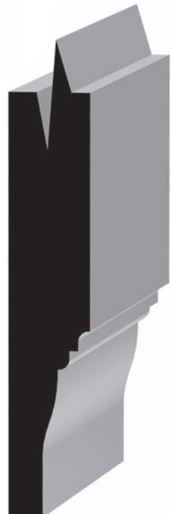
5/8" Panel with Small Bead & Cove Hip
