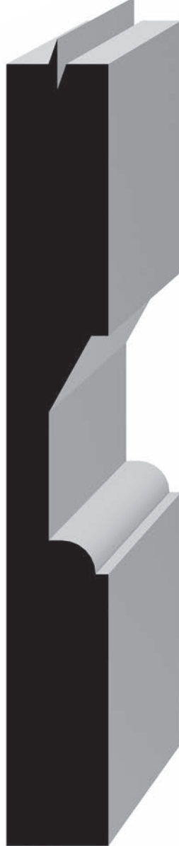
3/4" Thick Standard Raise with Quarter Round Sticking
