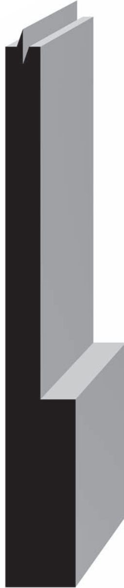
3/4" Thick Flat Panel with Square Sticking CNC Routed MDF
