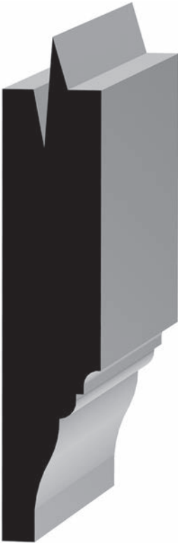
3/4" Panel with Small Bead & Cove Hip
