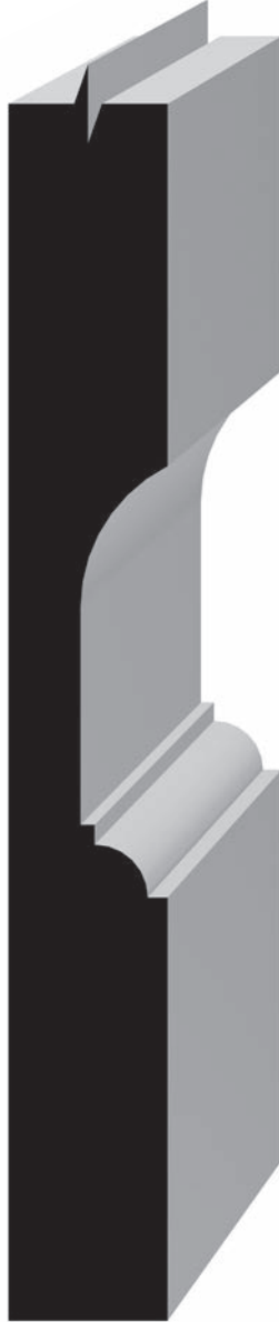
3/4" Thick Cove Raise with Ovolo Sticking
