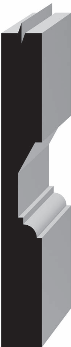
3/4" Thick Standard Raise with Ovolo Sticking
